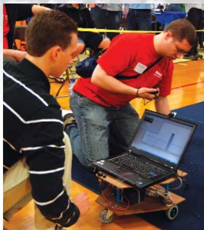
The Vision Centric Challenge (VCC) used a laptop-based robot named L2Bot that read a 2D barcode using an on-board webcam.
