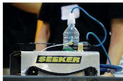
The members of senior team Homemade Titanium from Clawson, Michigan, researched landmines and designed SEEKER —a lightweight, low-cost, fully autonomous robot that searches for and marks the locations of landmines.
