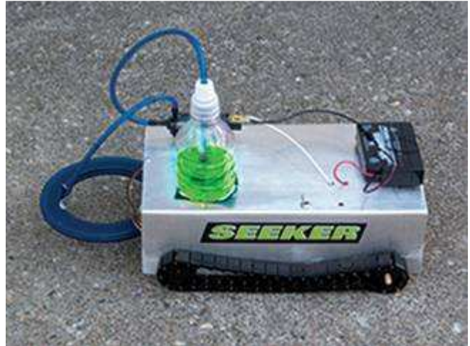
Figure 24. Seeker – landmine detection robot
