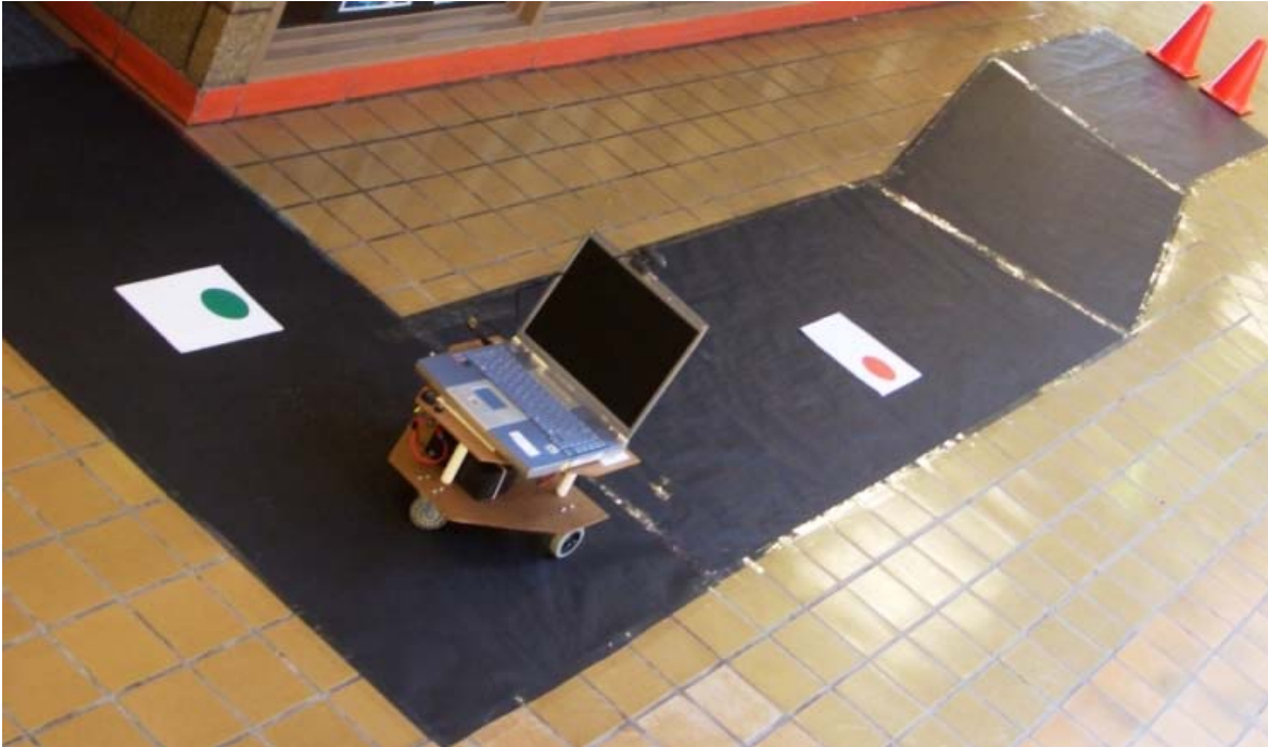
The robot started after recognizing the green light and is about to stop at the red light.
