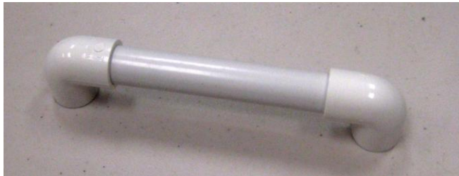
[Figure 4] Broken Pipe Assembly: 15cm pipe and two elbows
