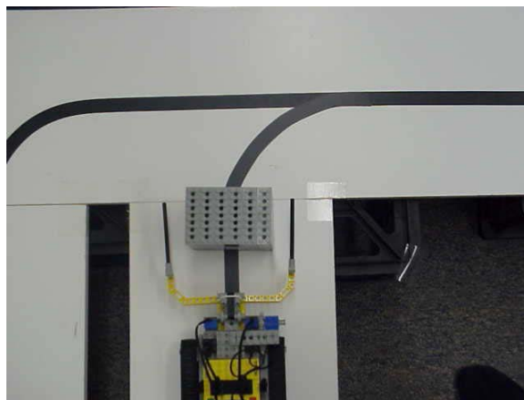
Fig. 8 A junction from the second base. A concrete barrier is located at the edge of the board. Any part of the second robot cannot pass the edge.
